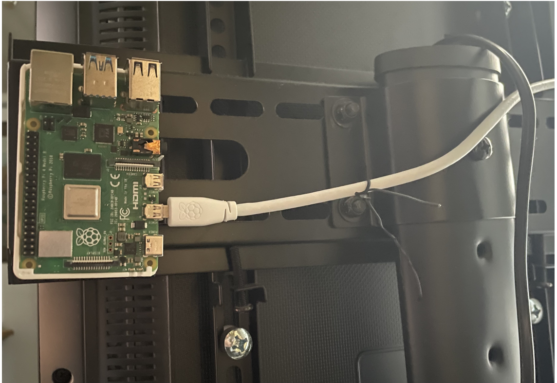
Figure 8. Raspberry Pi mounted behind a vertical display rack.
