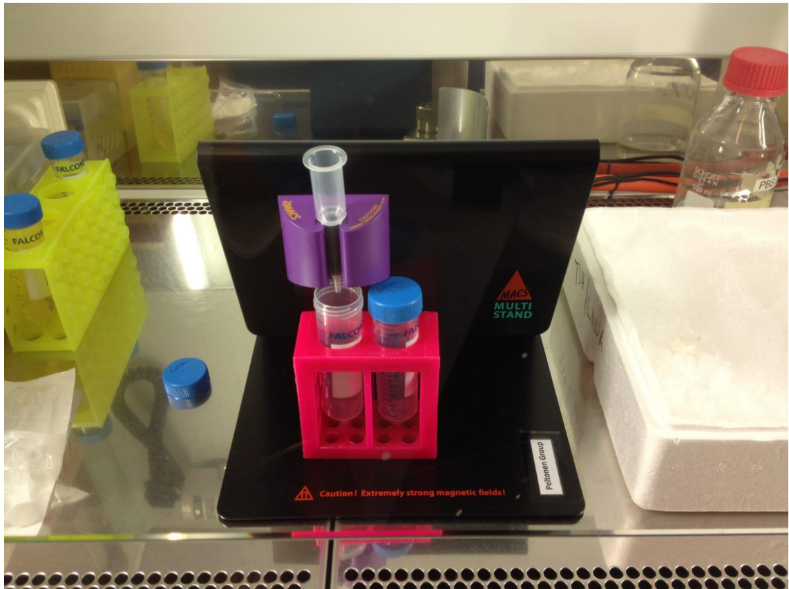
Figure 10. Picture taken during the laboratory work in this project. Image shows a multi-stand (black object) on which midiMACS magnet (purple object) is placed. Finally, the LS column is placed into midiMACS magnet. The setup was used to isolate the CD34+ or CD14+ cell fraction from PB-MNCs with specific magnetic beads.
