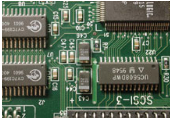
Figure 2.1: Surface mount components on a PCB.
