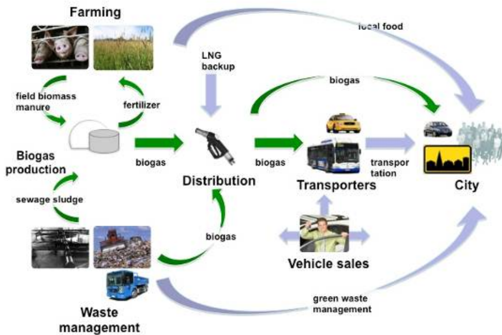
Figure 2. The biogas production and utilisation system
