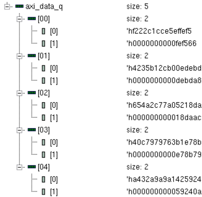
Figure 50: Screenshot of the reference queue and output queue for AXI writer unit
