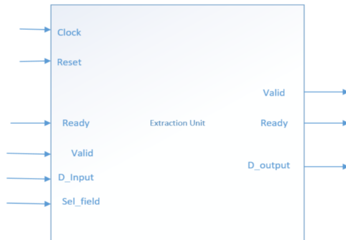
Figure 25: Extraction unit I/O interface
