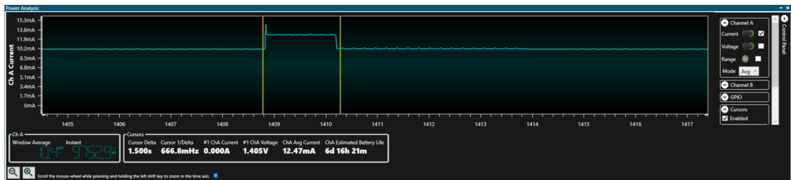
Figure D.14: Inefficient SW driver measurement time capture.
