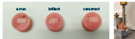
Figure 4. Illustration of different failure modes. Samples after SBS test, fractures were cohesive in all CAD/CAM composites and with glass-ceramic there were only adhesive fractures.
