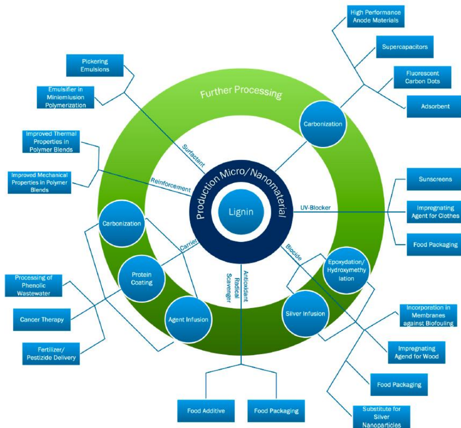
Figure 1.6 Overview of potential application of lignin-based micro- to nanoparticles. Reprinted with the permission of reference (Beisl et al., 2017).
