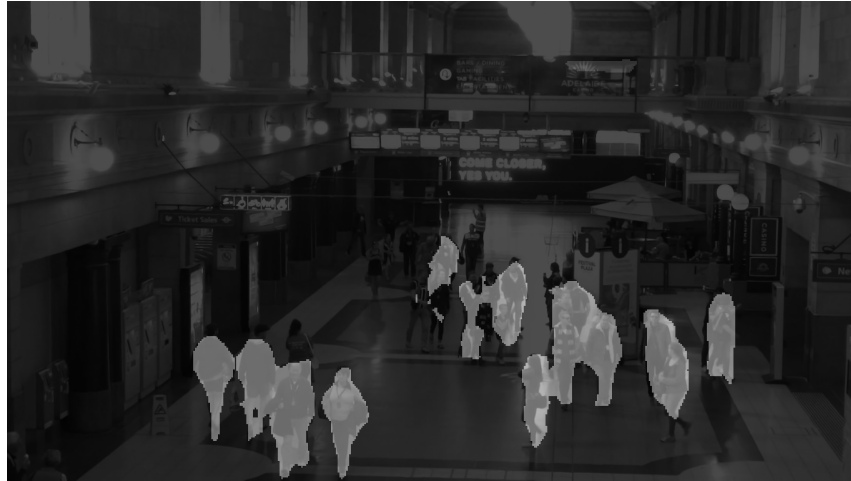
Figure 4.2: Semantic segmentation done to a picture. Every pixel is labelled as a person or as a background. [18]
