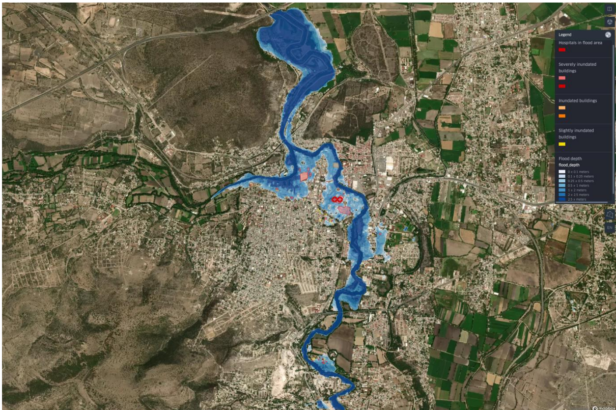
Figure 15. The flood map of Tula de Allende, Mexico created using Python. Creating this map does not need any user input apart from changing the file path to the raster of a flooding event and the WSF2019-Pop data.
