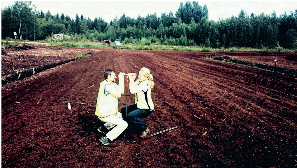
Figure 36.3. Determining the peat depth at the Kiihansuo mire in Savitaipale in July 2015. Professor Mika Lavento and Satu Koivisto applying a small 'Russian' peat corer. Photo T. Rostedt.
