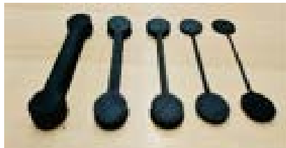
Figure 3: Graphene doped ABS samples prepared by YRP students with no materials science background.
