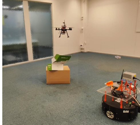
(b) Picture of the test environment while the MAV is hovering.
