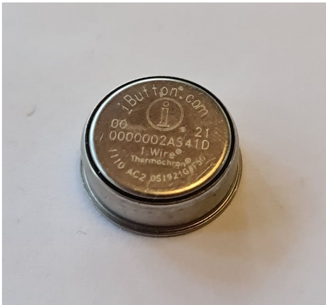
Figure 6. iButton Thermocron temperature loggers are small (diameter 18mm) and rugged temperature loggers suitable for multiple purposes.
