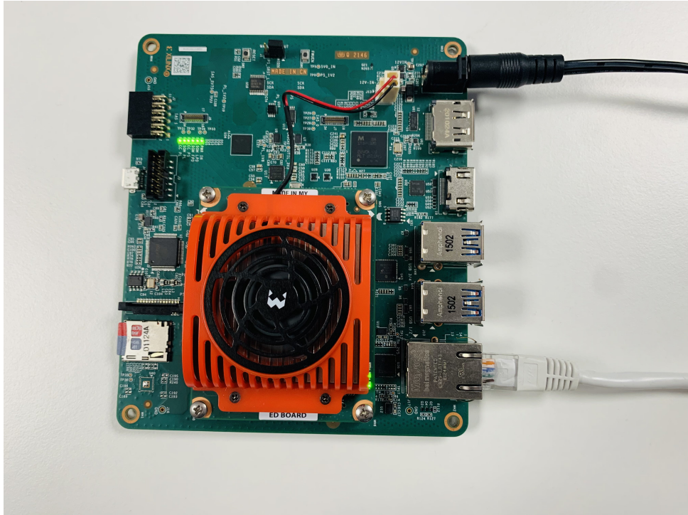
Figure 4.4: The Kria KV260 is used as an edge computing hardware accelerator.
