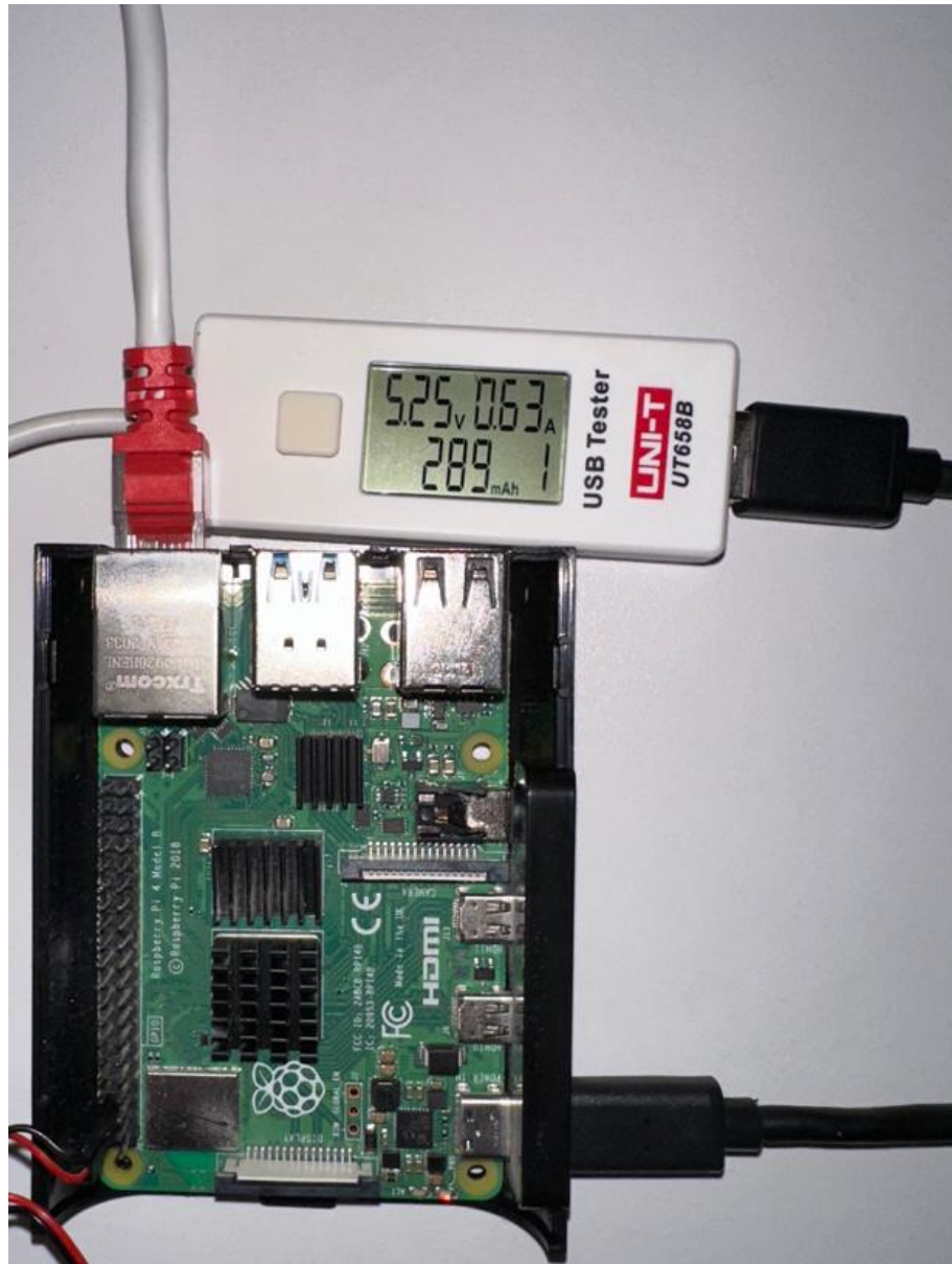
Figure 5.1: Measuring the power consumption of the Raspberry Pi with a USB tester.
