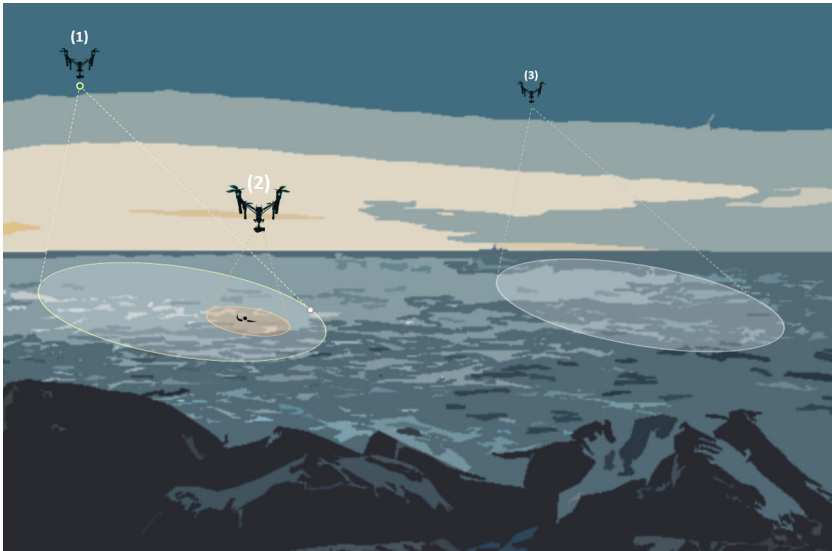
Figure 35. Illustration of active-vision-based search in maritime environments with UAVs. A single UAV can first fly higher to cover larger areas and descend in the event of a positive detection to increase reliability. Search time can then be optimized by dynamically adjusting the altitude depending on the perception confidence.
