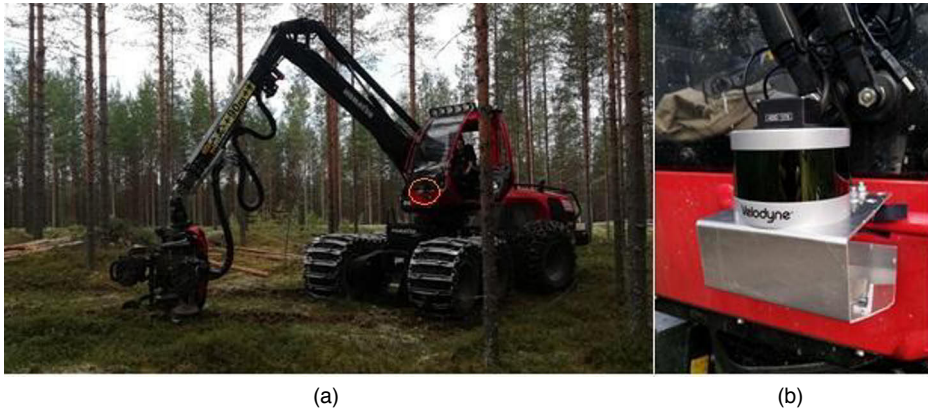
Figure 21. Sensor and harvester platform. (a) Komatsu Forest 931.1 forest harvester. The LiDAR scanner is marked by a red circle in the front of the windshield of the cabin. (b) A close-up of the LiDAR scanner.
