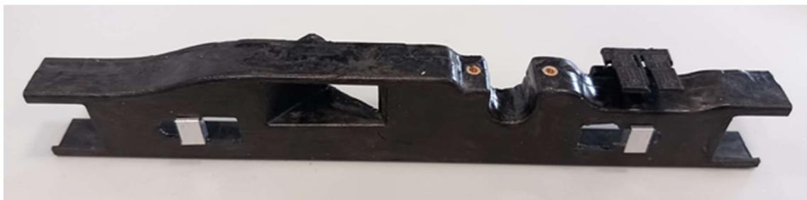
Figure 4 - Finished part with inserts, preheater connector clip and cooling pipe sleeve blocker.
