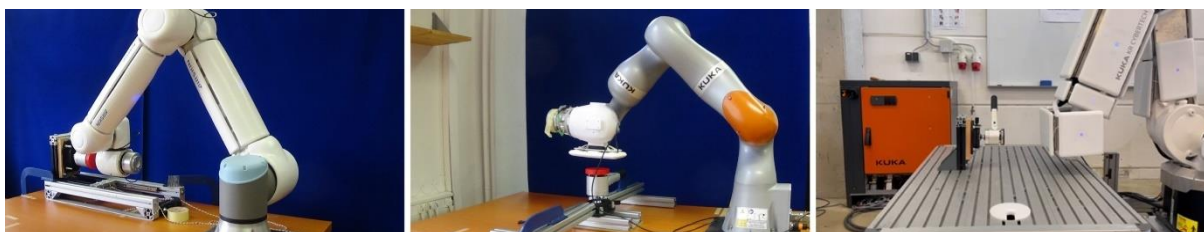
Figure 2: External soft skin safety covers on robotic manipulators and the experimental setup [12]. The soft skin can be recognized as the white cushioning on the cobots.
