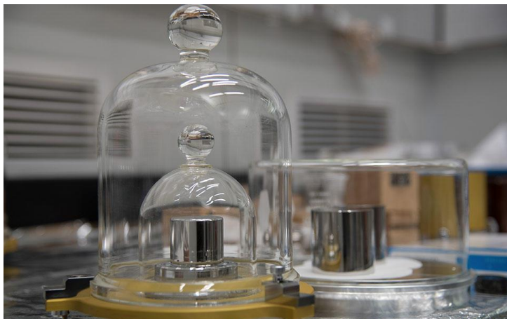
Figure 4 A reference standard for one kilogram from 1875 to 2018 [15]
