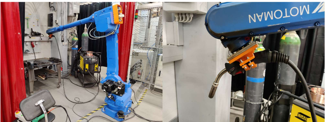
Figure 1 WAAM robot arm (left) and its MAG-welding type nozzle head (right) in Koneteknologiakeskus, Turku, Finland
