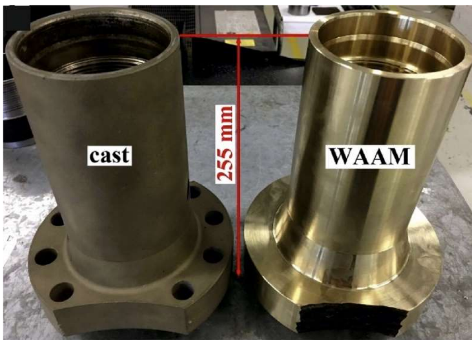
Figure 14 NAB-based part created with casting (left) and WAAM (right, post-processed) [15]
