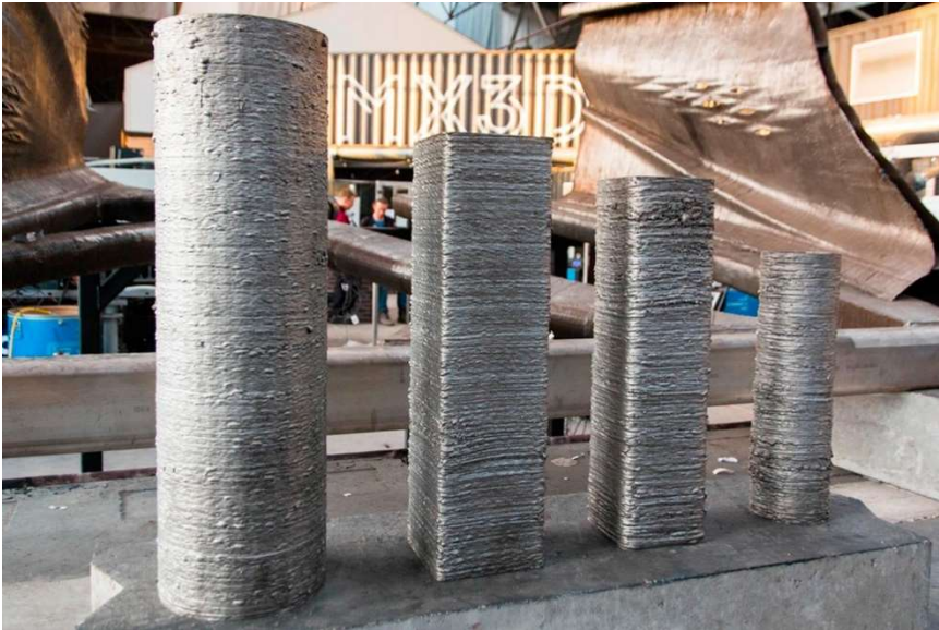
Figure 9 Circular and square hollow tubes created from stainless steel with WAAM [6]
