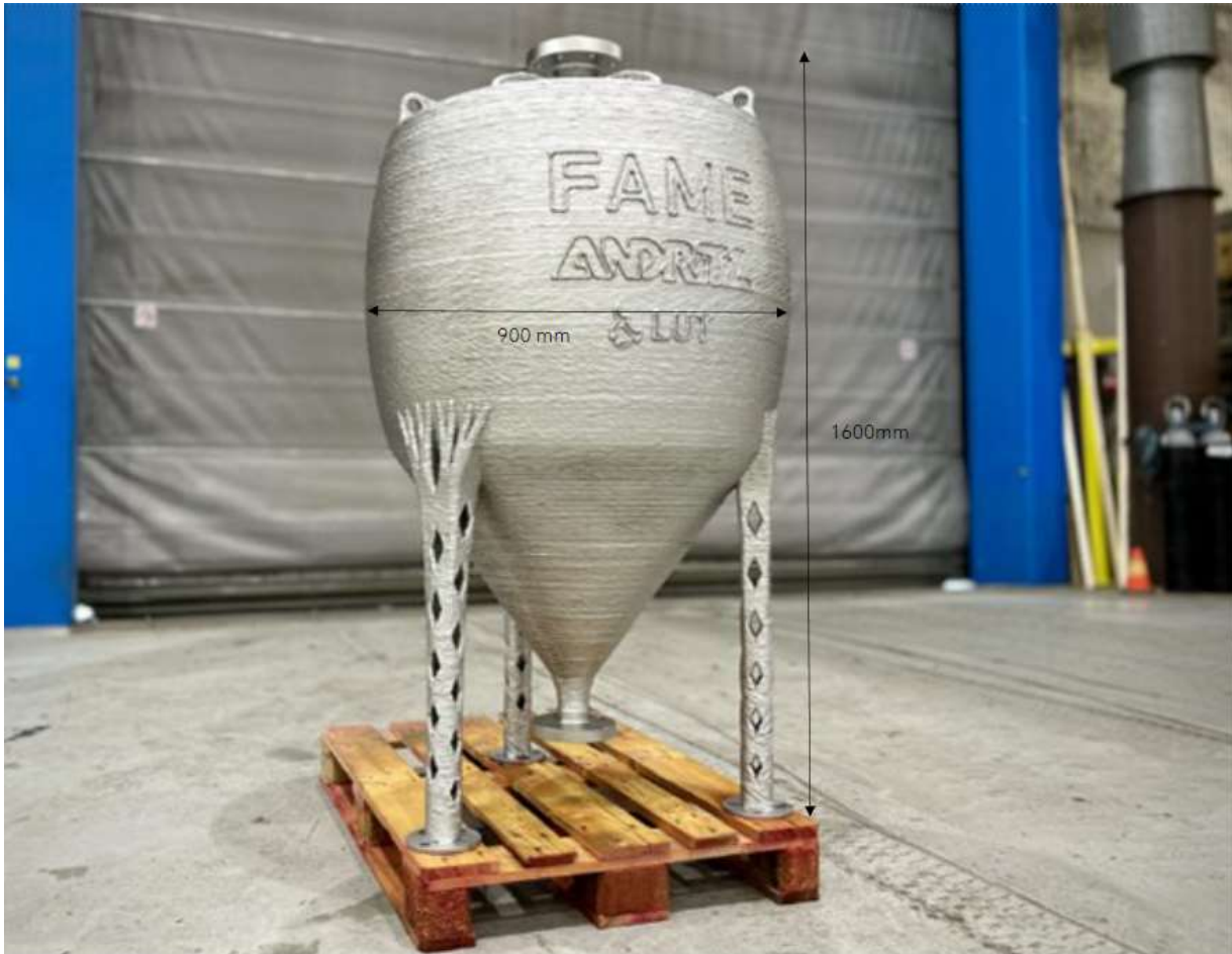
Figure 10 Pressure vessel created by Andritz Savonlinna works oy and FAME [14]
