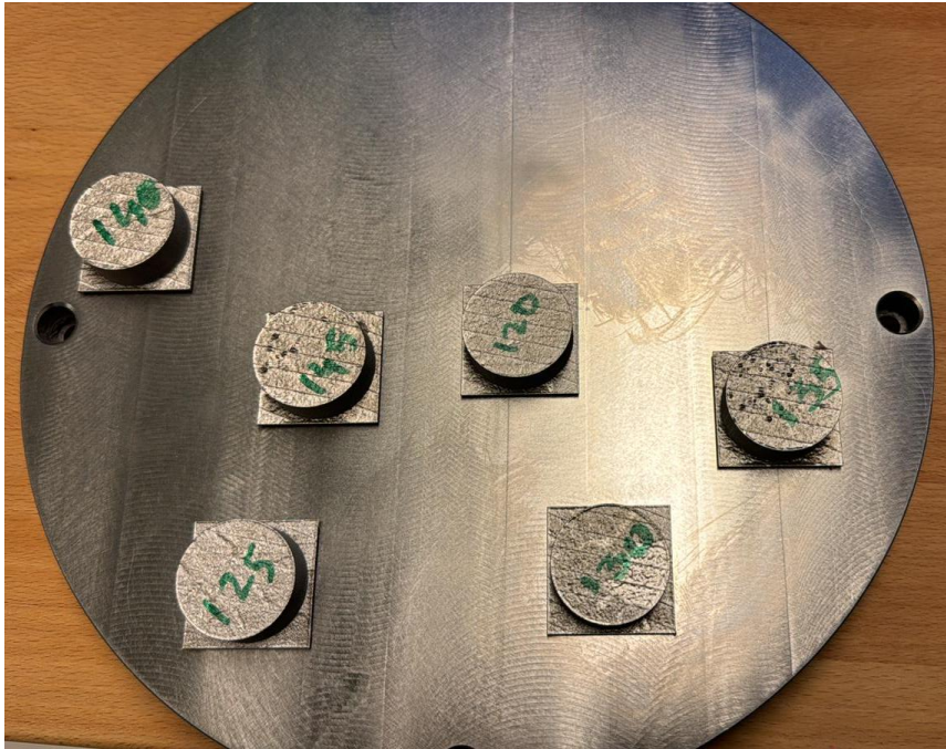
Figure A 2. As-built NiFDSS samples after the second trial of process parameter optimization.
