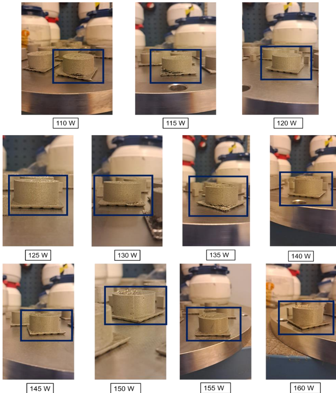
Figure 34. As-built NiFDSS specimens manufactured with varying laser power from 110 W to 160 W. Based on the observation of the first trial, for the second attempt, samples were fabricated with laser power from 120 to 145 W. During the second attempt between 120 W to 145 W, it was observed that cracks disappeared after 135 W, indicating that the optimal power range lies between 135 W to 145 W. Cracks were observed in samples processed at 120 W, 125 W, and 130 W. Therefore, the conclusion was in alignment with the first attempt.
