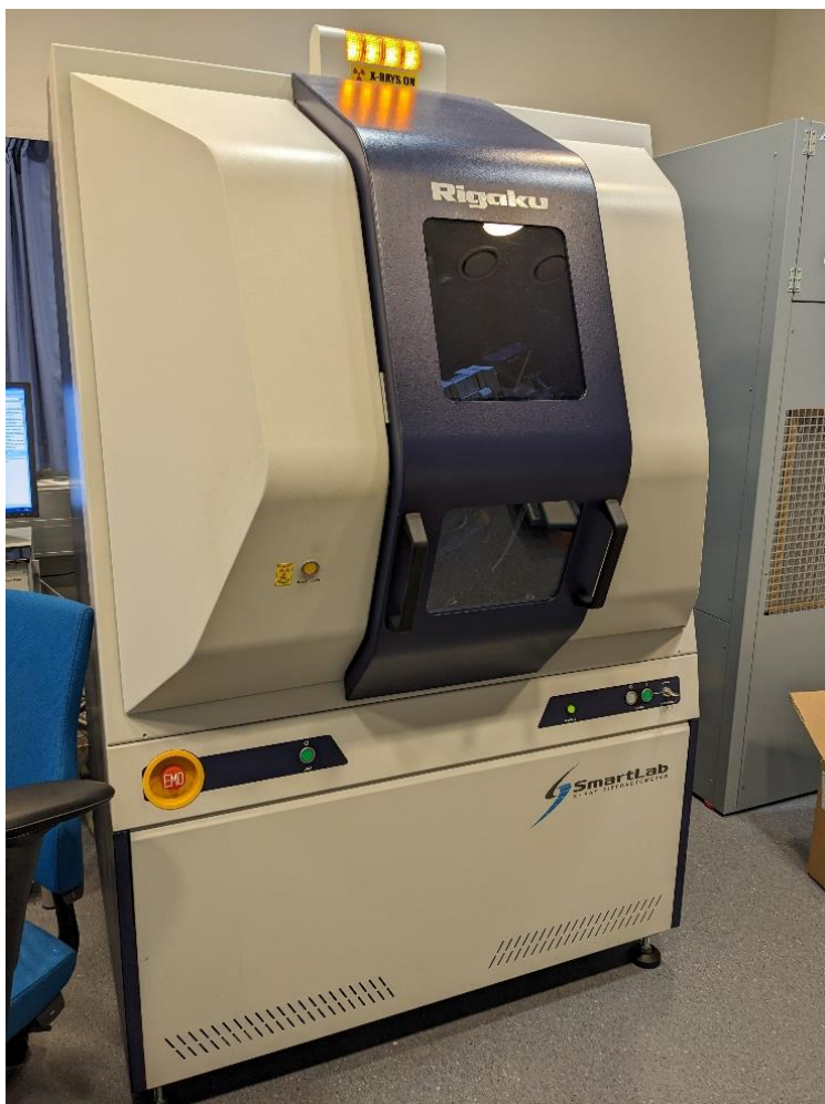
Figure 12: Rigaku SmartLab 9 kW XRD machine.
