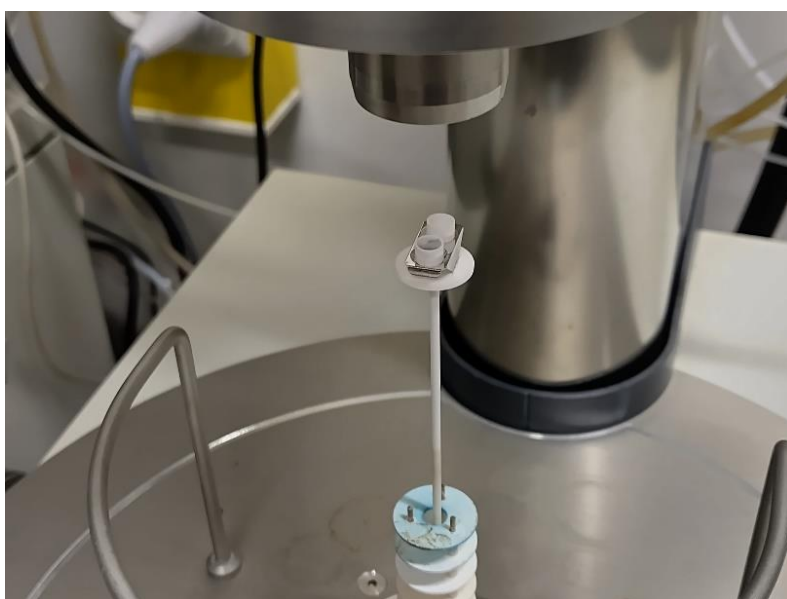
Figure 22: Crucibles for reference and sample used in DSC-TGA-MS experiment.
