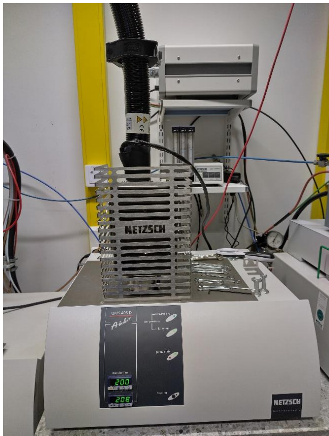
Figure 21: NETZSCH QMS 403 D Aeolos machine for DSC-TGA-MS experiment.
