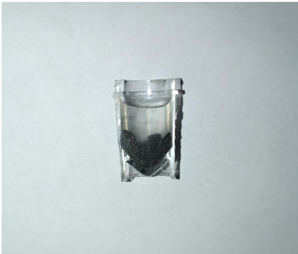
Figure 18: One part of the cut V-vials including a sample mixed with resin.
