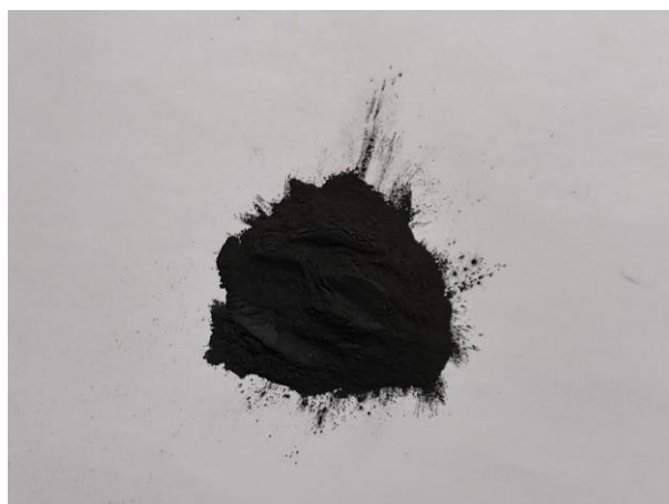
Figure 9: Black mass attained after the pre-processing stage.
