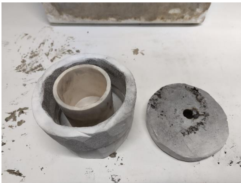
Figure 24: Alumina crucible used in the experiment.
