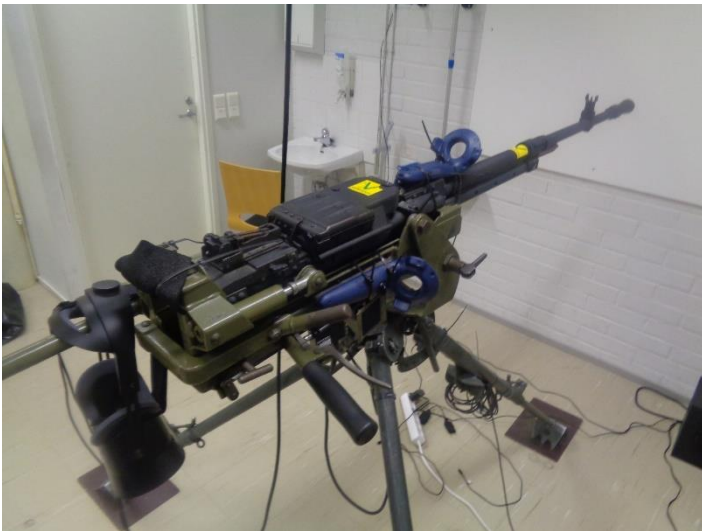
Figure 11. Top View of the New VR-based Simulator with VR Glasses. Picture: Elias Lehtonen.
