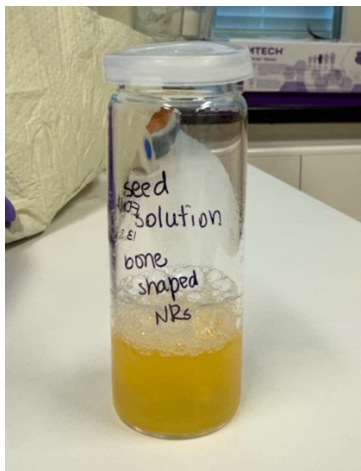
Figure 7. Seed solution for seeding method for synthesis of bone-shaped Au NRs.
