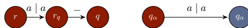
Figure 12. A transition graph on the left side represents a sub-routine, which replaces each instruction (r, -, q) of \mathcal{M}_R^- , where r \neq q'_\alpha . The transition graph on the right side represents the transition from \mathcal{M}_R^- to \mathcal{M}_R^+ at the state q_\alpha . Here a \in \Gamma' .
