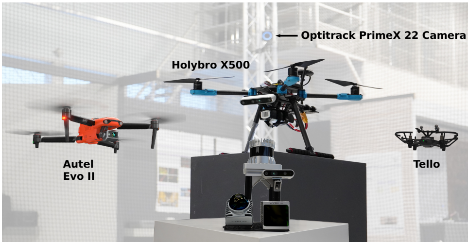
Figure 19: Illustration of the hardware used in the experiments. At the bottom, the tracking sensors including Ouster OS1-64, Livox Mid-360, Livox Avia and Intel RealSense D435.
