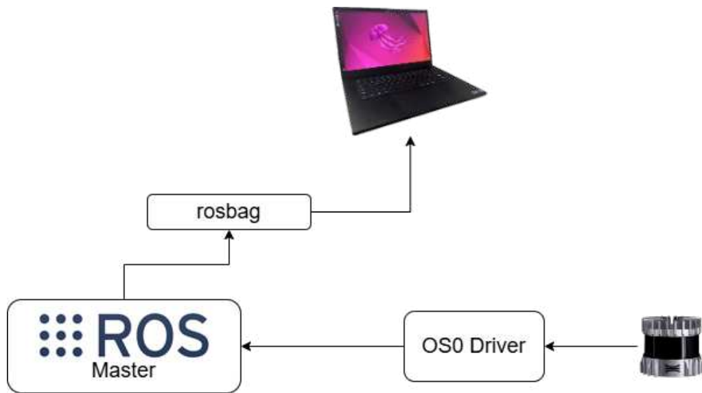
Figure 2.3: ROS interfaces for the LiDAR sensors integrated
