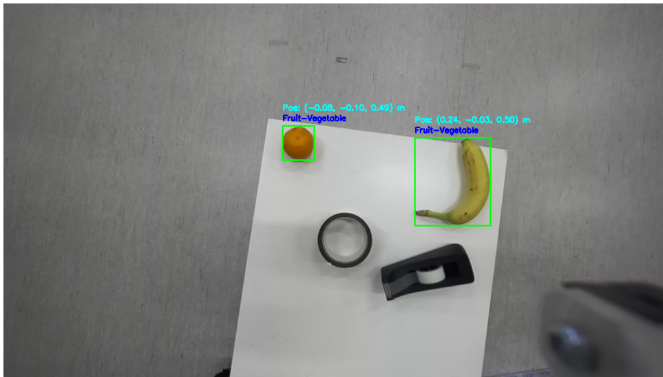
Figure 3.3: Fruit detection and 3D position estimation using the ZED SDK.
