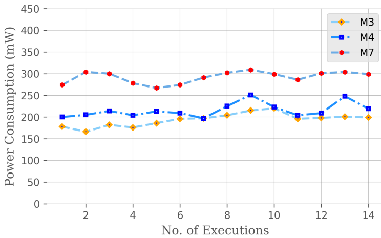
Figure 28: Average power consumption during ECDSA implementation using STM32F427 M series processors
